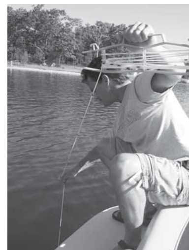
Jim Dixon, CLMP volunteer, slowly lowers a Secchi disk into the water in order to make a lake transparency measurement. photo: HRWC
