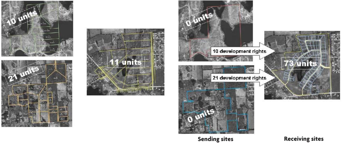
Figure 1-1. Parcels in Highland Township, Michigan identified as hypothetical sending and receiving sites. Without TDR (left), three sites are developed on 433 acres producing 42 units, while with TDR (right), one site is developed on 125 acres yielding 73 units as a result of development right transfers. A 2:1 allocation rate is employed resulting in one development right created in a sending site is two rights that can be transferred to a receiving site.
