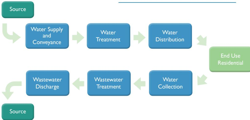
A simplified water use cycle. Energy is used in most of the steps of the water cycle. Modified from California Energy Commission, 2005 Integrated Energy Policy Report.
