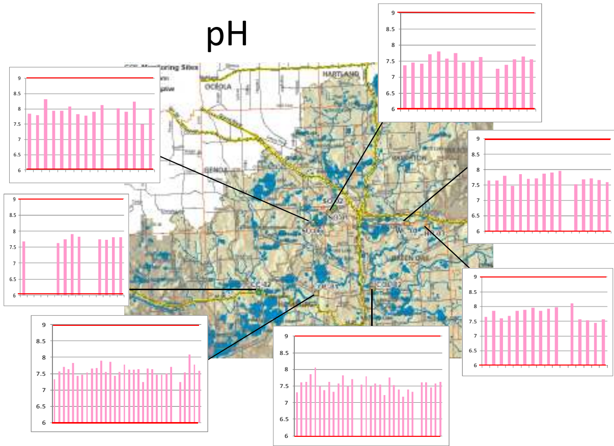
Figure 6. pH levels recorded at long-term monitoring sites, with state water quality standards indicated by red lines.
