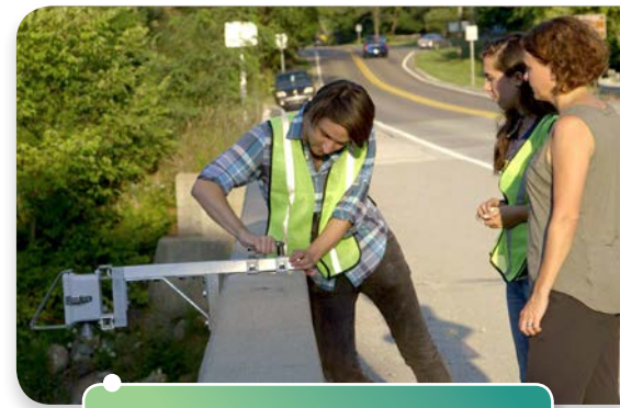
University of Michigan students installing low cost water level sensors to help dam operators manage flows.
