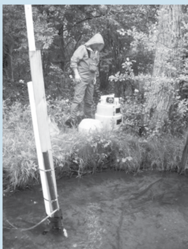
The autosampler being set up as a storm rolls in at Honey Creek. The intake hose is attached to the water level logger in the foreground. photo: HRWC
